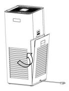
2> To unlock the filter lock: Hold the filter lock block and pull it out. When pulled out, the filter unlocks and descends.
