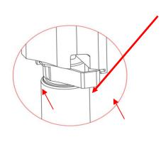
6> Load the new H13 filter: Place the new H13 filter on the locking tray. (Note: It is necessary to put filter with the pull tab towards to the user)
